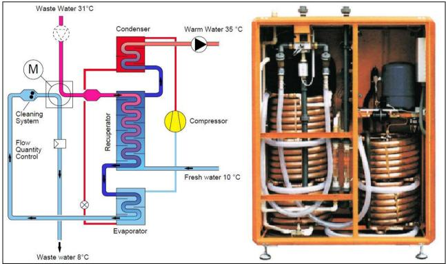
Fig.3 Waste water heat recovery unit with recuparator and heat pump
