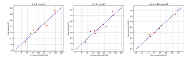
**Fig. 8** Correlation between the solar heat gains resulting from the heat balances performed separately in both units, and the solar irradiation measured on a vertical plane parallel to the façade, for insulated units A (left) and B (middle) and correlation between the solar heat gains of both units (right).
