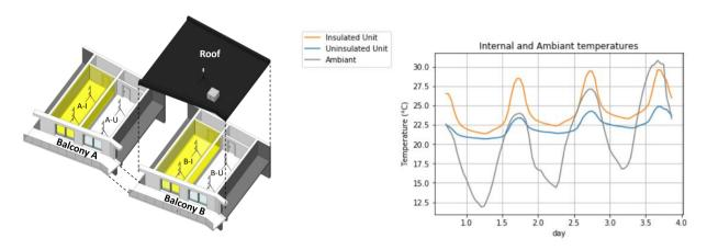
**Fig. 3** Measured floating temperatures with and without insulation panels covering the party walls of identical units (Printemps, Brussels, 2017/05/24-2017/05/27).
