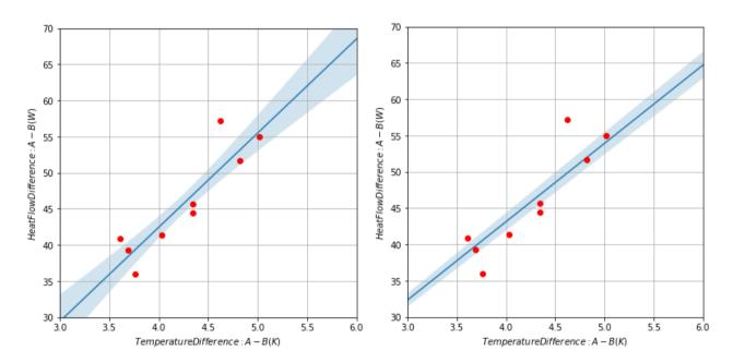
**Fig. 7** Correlation between daily mean heat power differences and temperature differences between two identical insulated units, without (left) and with (right) forced intercept.
