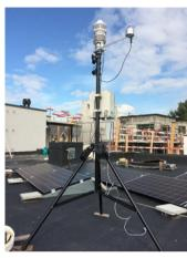
Fig. 1 Measurements sites: student dwellings in Etterbeek (up left), apartments in Neder-over-Heembeek, Brussels (up right), experimental setup inside the units with insulation panels, electric radiator, internal air temperature sensors and external pyranometer on the balcony (down left), weather station located on the roof (down right).
