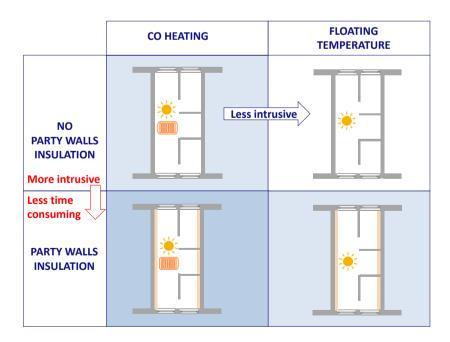
Fig. 2 Different boundary conditions and heat sources for the measurement of the Heat Loss Coefficient.
