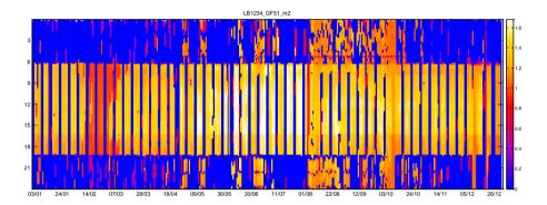
**Fig. 8** Carpet plot of supply air flow  $l/(s \cdot m^2)$  for all AHUs. The hours of the day according to the left-hand side scale are shown as a function of the days of the year.
