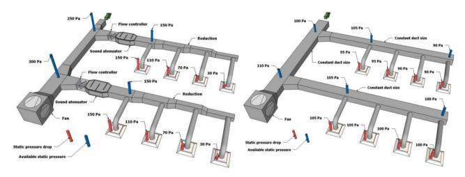
**Fig. 1** Ductwork sized with the constant pressure drop method (left) and ductwork sized with the final pressure drop method (right). [3]
