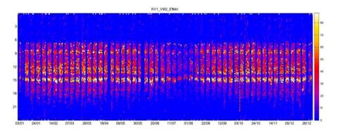
**Fig. 3** Carpet plot of heating power (kW), calculated from measured water flow and temperature assuming the incoming cold water is at  $+10^{\circ}$ C, for domestic hot water colour-coded according to the right-hand side scale. The hours of the day according to the left-hand side scale are shown as a function of the days of the year.
