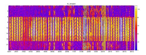
**Fig. 7** Carpet plot of building auxiliary electricity power (kW) colour-coded according to the right-hand side scale. The hours of the day according to the left-hand side scale are shown as a function of the days of the year.
