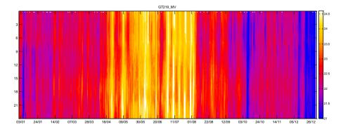
**Fig. 9** Carpet plot of landscape office indoor air temperature at the top floor. The hours of the day according to the left-hand side scale are shown as a function of the days of the year.
