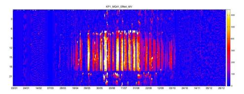
**Fig. 5** Carpet plot of the purchased district cooling power (kW) colour-coded according to the right-hand side scale (blue means a power close to 0 kW, white means a power of more than 600 kW). The hours of the day according to the left-hand side scale are shown as a function of the days of the year.
