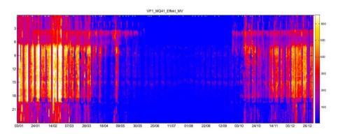
**Fig. 2** Carpet plot of purchased district heating power (kW) colour-coded according to the right-hand side scale (blue means a power close to 0 kW and white means a power over 600 kW). The hours of the day according to the left-hand side scale are represented as a function of the days of the year. Domestic hot water energy use is included in district heating energy use. Ground heating energy use is included in district heating energy use, but not in BBR requirements.
