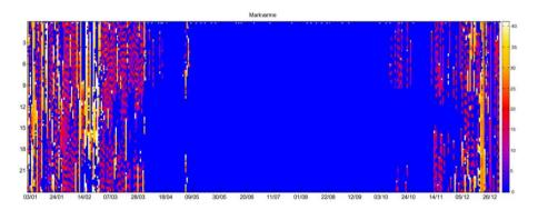
**Fig. 4** Carpet plot of ground heating power (kW) colour-coded according to the right-hand side scale. The ground heating system is turned off during blue periods (outdoor air temperature higher than +3°C). The hours of the day according to the left-hand side scale are shown as a function of the days of the year.
