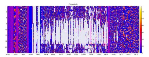
**Fig. 6** Carpet plot of the process cooling power (kW) colour-coded according to the right-hand side scale. Comfort cooling, faulty and missing measurements are coloured grey. The hours of the day according to the left-hand side scale are shown as a function of the days of the year.
