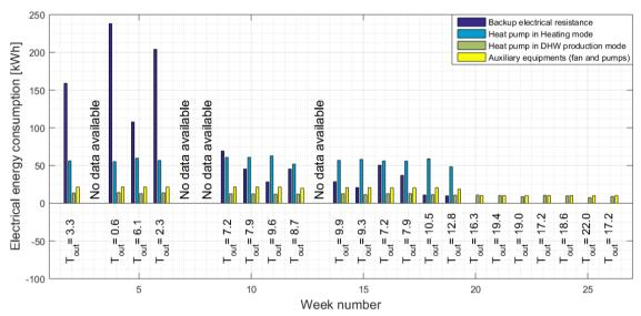
**Figure 5**: Electrical energy consumption of the backup electrical resistance, the heat pump in heating mode, the heat pump in DHW production mode and the auxiliary equipment on a weekly basis
