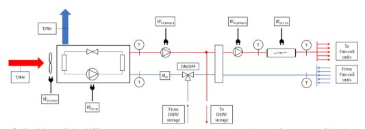
Figure 2: Position of the different sensors used to measure the on-site performance of the heat pump
