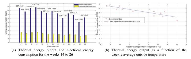
Figure 3: On-site performance of the heat pump in domestic hot water production mode
