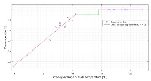
Figure 6: Coverage factor of the heat pump as a function of the weekly average outside temperature
