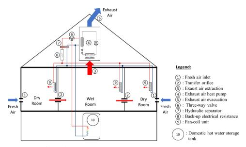
**Figure 1**: Simplified representation of the HVAC systems
