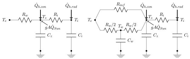
(c) RC circuit of second order: Zone and Internal temperatures. (d) RC circuit of third order: Zone, Wall and Internal temperatures.
