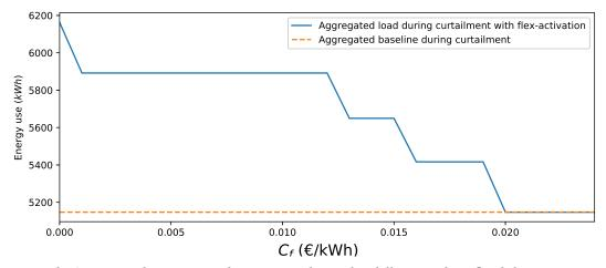
Figure 3: Aggregated energy use during curtailment for different values flexibility activation cost
