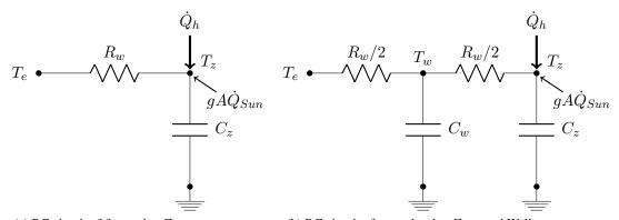
(a) RC circuit of first order: Zone temperature. (b) RC circuit of second order: Zone and Wall temperatures.
