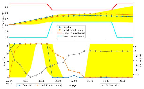
Figure 5: Zone temperature and load evolution of a building agent modelled with three states: Zone, Wall and Internal
