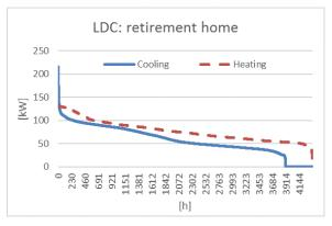
Figure 2: Heating (dashed line) and cooling (solid line) load duration curves.
