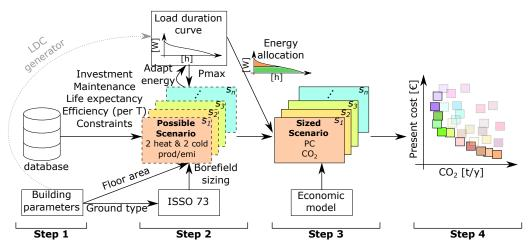
Figure 1: Schematic representation of the optimal Heating, Ventilation and Air-Conditioning (HVAC) design methodology split in four consecutive steps. The generation of load duration curves (LDC) based on a limited set of building parameters is not yet implemented and is therefore represented as a dotted grey arrow.
