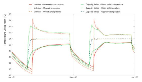
**Fig. 4** Time series data for capacity limited HVAC system with early start-up versus unlimited power (semi-detached heavyweight dwelling with R5 insulation, standard double glazing and medium glazed area)
