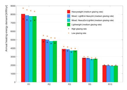
**Fig. 2** Annual space heating demand in relation to thermal insulation, building thermal inertia and window size for buildings with standard double glazing and intermittent thermostat schedule.
