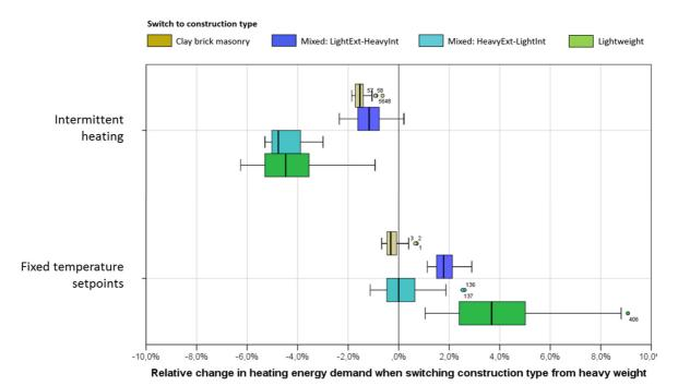
**Fig. 3** Relative change in annual heating demand when switching construction type from heavy weight to different variants with less thermal inertia – in relation to distinct heating schedules.
