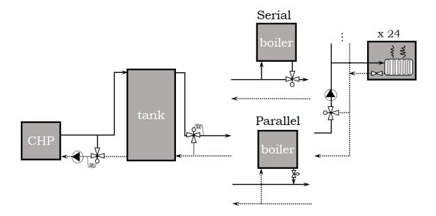
Figure 1: Schematic representation of two hydronic designs: a serial and a parallel connection of the boiler.
