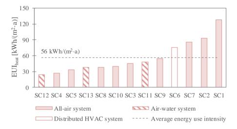
Fig. 5 Average annual heating energy use intensity (EUI<sub>heat</sub>) of the shopping centers from 2012 to 2014.
