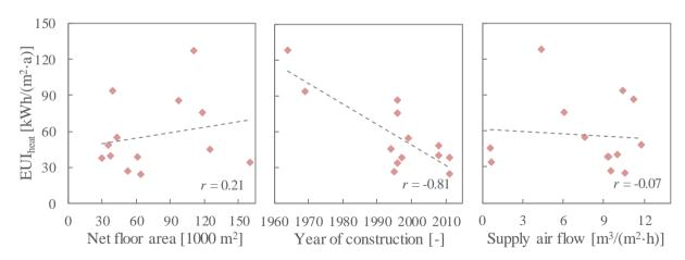
**Fig. 6** Heating energy use intensity (EUI<sub>heat</sub>) of the shopping centers as related to the net floor area (left), the year of construction (middle) and the specific supply air flow rate (right).
