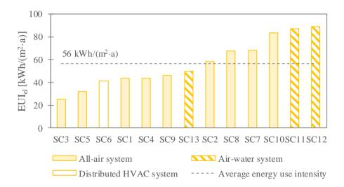
Fig. 2 Average annual electricity use intensity (EUI<sub>el</sub>) of the shopping centers from 2012 and 2014.
