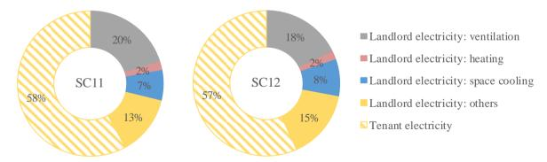
**Fig. 4** Breakdown of the total electricity use in SC11 (left) and SC12 (right) based on the measured data from 2012 to 2014.
