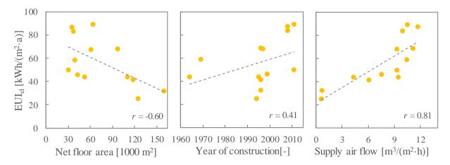
**Fig. 3** Electricity use intensity (EUI<sub>el</sub>) of shopping centers as related to the net floor area (left), the year of construction (middle) and the specific supply air flow rate (right).
