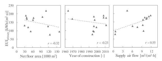
**Fig. 8** Primary energy use intensity (EUI<sub>primary</sub>) of the shopping centers as related to the net floor area (left), the year of construction (middle) and the specific supply air flow rate (right).
