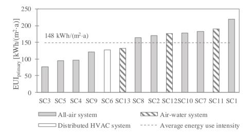
Fig. 7 Average annual primary energy use intensity (EUI<sub>primary</sub>) of the shopping centers from 2012 to 2014.
