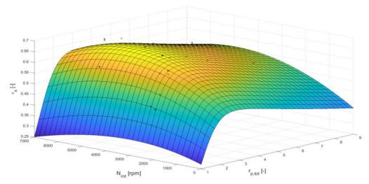
Fig. 5 Isentropic efficiency surface.
