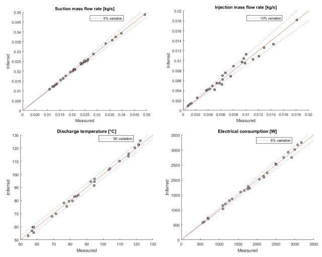
Fig. 4 Compressor model parity plots.
