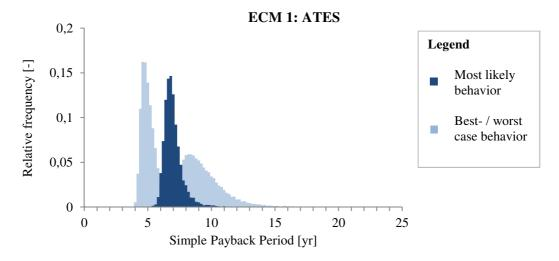
**Fig. 6** Predicted Simple Payback Period of an ATES system based on best case, worst case and most likely occupant behavior.
