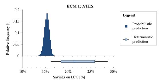
**Fig. 5** Comparison of the probabilistic- and deterministic approach for predicting the savings on Life Cycle Costs of an ATES system.
