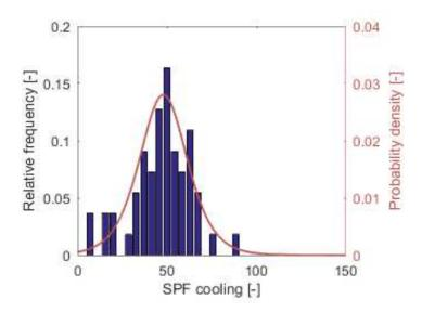
**Fig. 4** Histogram plot of the acquired field data (blue columns) and corresponding probability density function (red line) for the SPF-cooling of ATES systems.
